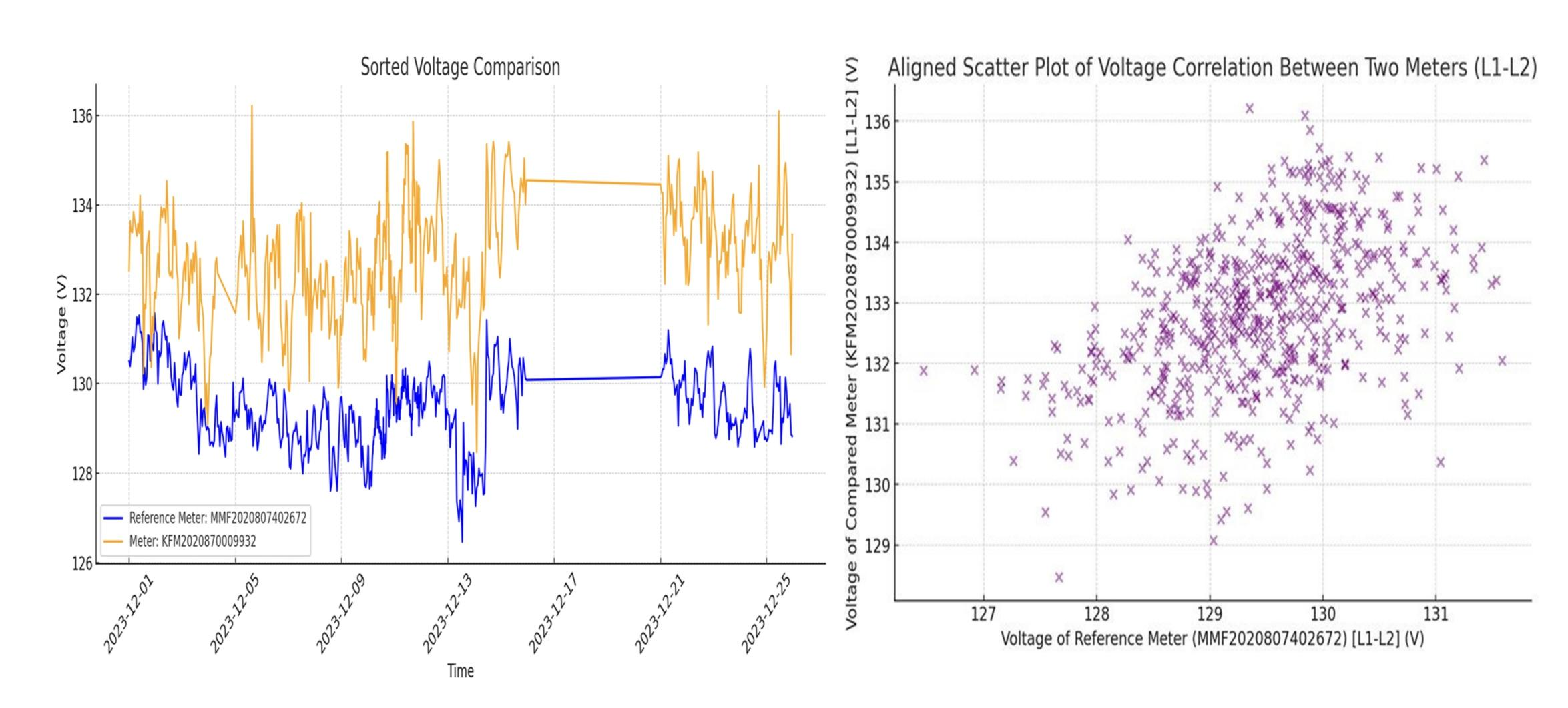
As depicted here, diverging voltage trends and non-correlated scatter points indicate an absence of expected connectivity. These anomalies were flagged by the AI/ML model for further validation and correction, showcasing its ability to identify and address inconsistencies within the distribution network.
